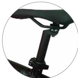
4. Orient the seat and tighten the seat post correctly using the seat collar on the frame (photo on the right). **Do not raise the seat tube beyond the limit indicated on the seat post to avoid breaking the frame and serious injuries while riding.**
