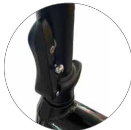
3. Position the handlebar stem in a vertical position, then tighten the handlebar using the specific lever on the handlebar stem.
