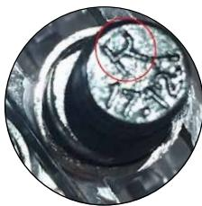
5. Identify the right pedal by the R mark on the pedal axle, while the L mark identifies the left pedal.
